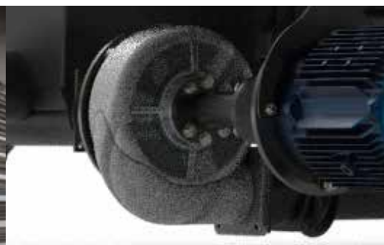
Rinsing out sediments via centrifugal pump
