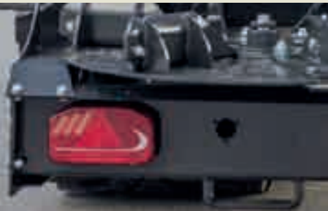
„Dynamic“ full-LED rear light with dynamic indicator made from impact-resistant material
