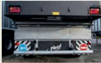
Germany 40 km/h version with fixed underride guard
