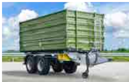
TDK 160 with 1800 mm body (3 x 600 mm tailgate)
