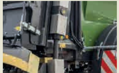
Milling drum drive above drive shaft
