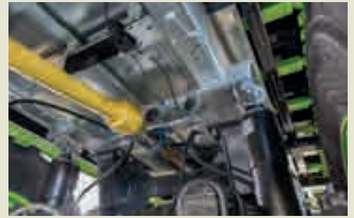
On KDS tandem and tridem: chassis guard (manure protection)
