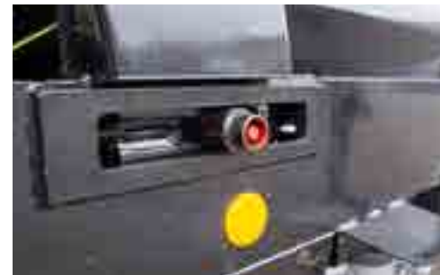
Easily accessible chain wheels which can be lubricated through the shaft on either side
