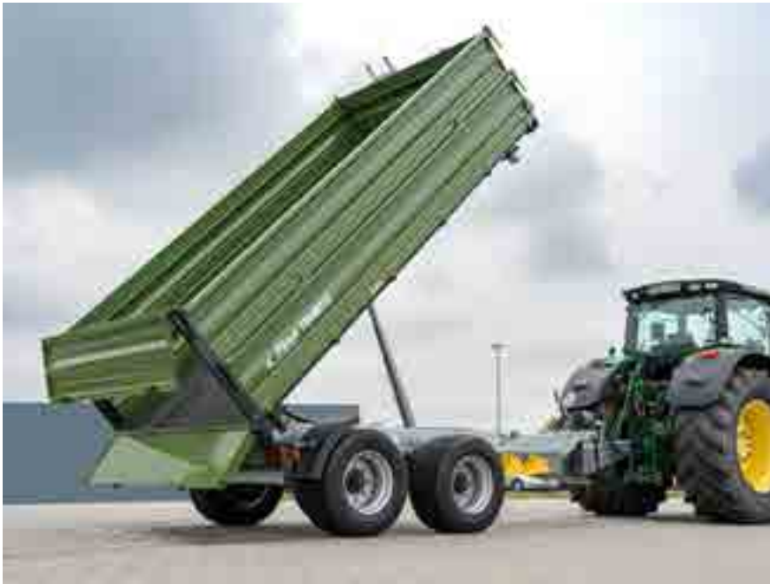
TDK with hydraulic gravel flap 500 mm
