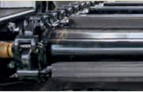
Forged chain links with 20 mm diameter and a breaking load of 50 t along with solid conveyor strips that are closed at the top and spaced at 300 mm intervals to ensure even and reliable transport of even the heaviest of materials.
