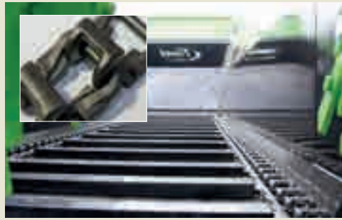
Forged chain links with 20 mm diameter and a breaking load of 50 t along with solid conveyor strips that are closed at the top and spaced at 300 mm intervals to ensure even and reliable transport of even the heaviest of materials.
