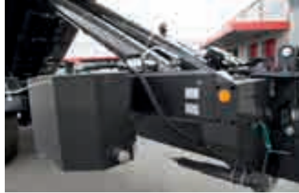
On-board hydraulics 60 litre (optionally 90 l) driven by PTO shaft with hydraulic pump and oil container
