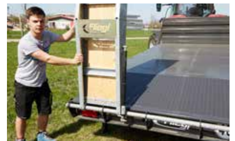
Practical: movable drive-on segments to adapt to track width
