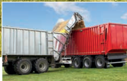
“MobilFast” overloading belt (up to 30m 3 /min)
