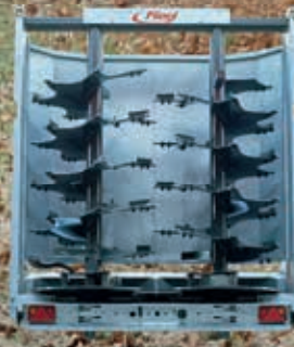
Milling drums with slingers
