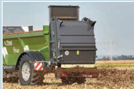
Spreading widths of up to 32 m are possible with the varioSPLASH wide disc spreader.
