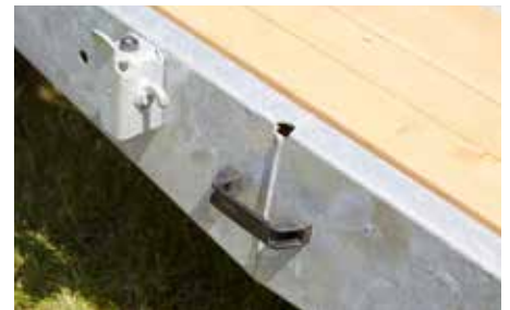
Drive-on ramps with wood covering, bridge floor made of 3.5 mm steel sheet, painted on the TPA 120
