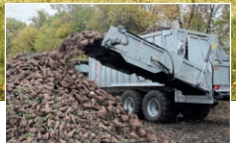
RUBY overloading belt for sugar beet Overloading rate approx.: 15m 3 /min
