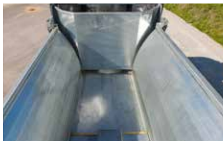
Minimum wear with hydr. pushing system - no scraper floor.
