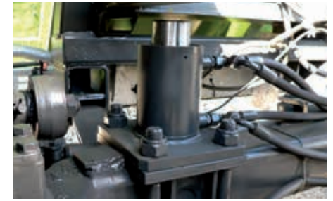
Optional: hydraulic support at the axle
