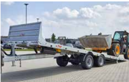
From TPA 200 on: Hydraulic tipping drawbar
