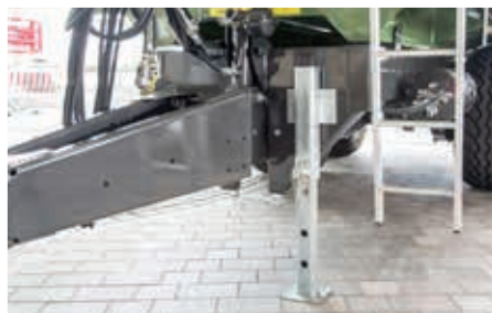
standard starting from TMK 256: hydraulic drawbar suspension and drop support leg, mechanical
