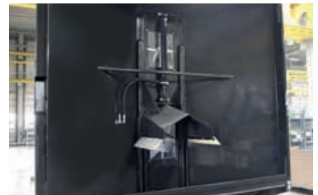
Hydr. sliding gate allows the overloading auger to be completely emptied when loaded
