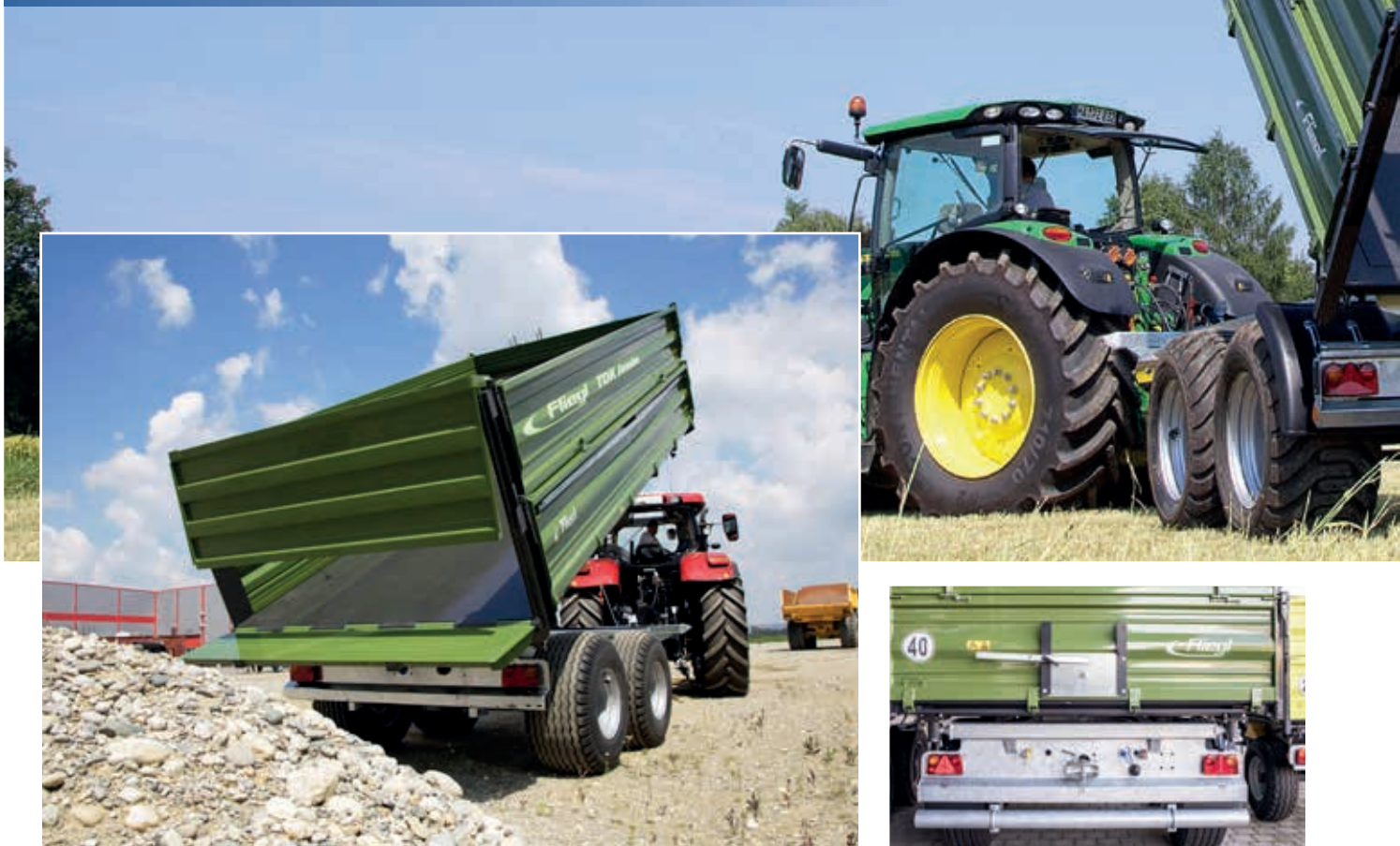
TDK 160 with hydr. gravel flap 500 mm Bridge: 5000 x 2320 x 2220 mm
