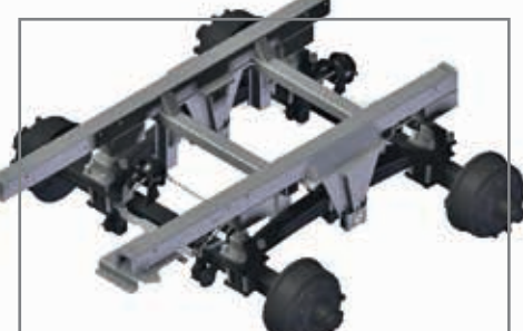
Titan tandem assembly for best ground compensation.
