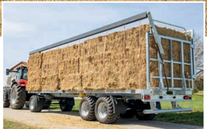
DPW 210 Ultra with closed load securing. Opening is possible on the right or left.
