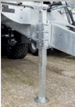
Hydraulic supporting leg
