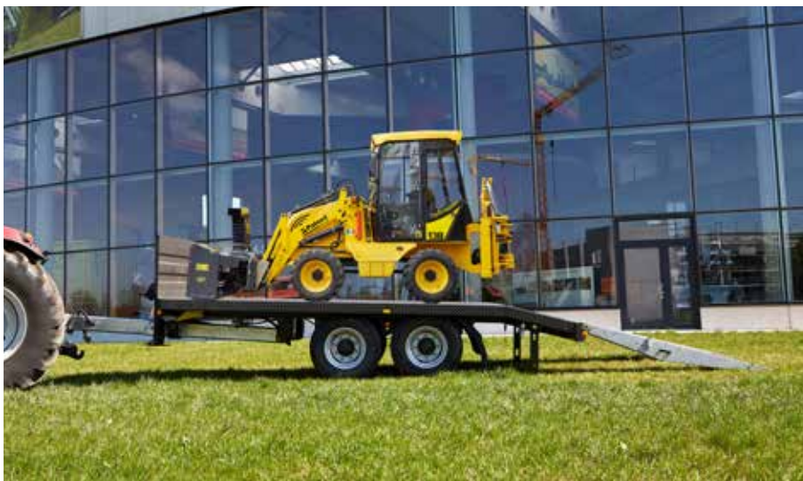
Practical: movable drive-on segments to adapt to track width
