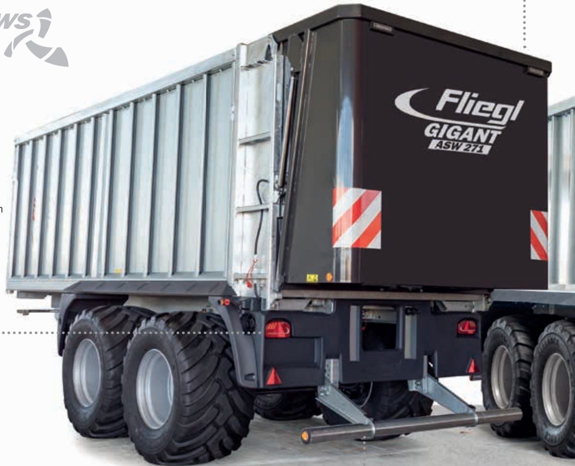
Full LED rear lights with dynamic indicator made of impact resistant material.
