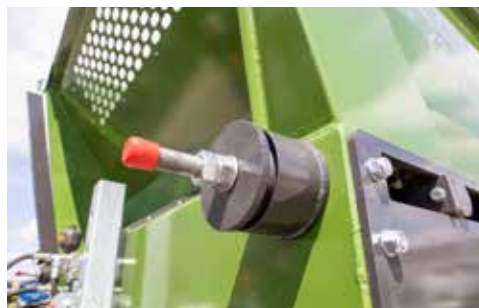
Mechanical chain tensioning
