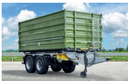
TDK 160 with 1800 mm body (3 x 600 mm tailgate)
