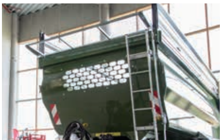
Mechanically folding protective grating
