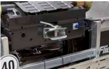
Optional: extendible lighting carrier, brake connection and hydraulics for 2nd trailer
