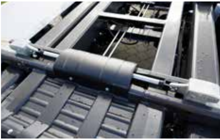
Reversible locking system for inside and outside locking
