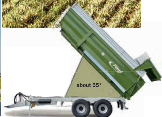
Tandem TMK 269 Profi with body length 6.90 m and tilt angle about 55°
