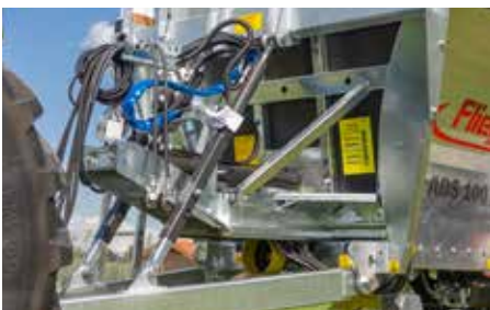
Hydraulic drawbar suspension, best ride comfort
