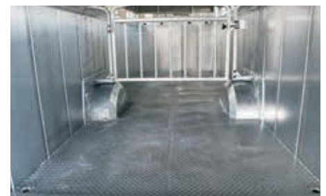
Chequer plate floor for animal safety
