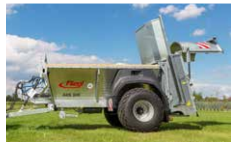
Hydraulic sliding gate
