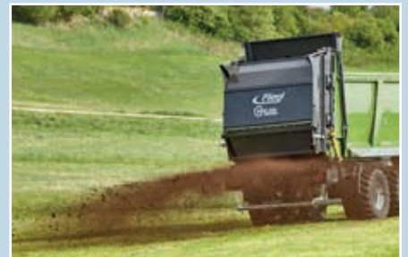
Spreading widths of up to 32 m are possible with the varioSPLASH wide disc spreader.
