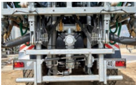
Fliegl SKATE 210 with pendulum frame for better slope compensation (only on SKATE 210/240)
