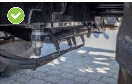
Centrally mounted axle, hydraulic steering for crab steering mode
