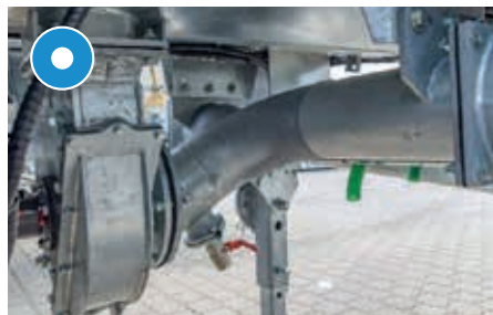
Hydraulic turbo filler, centrally under tank
