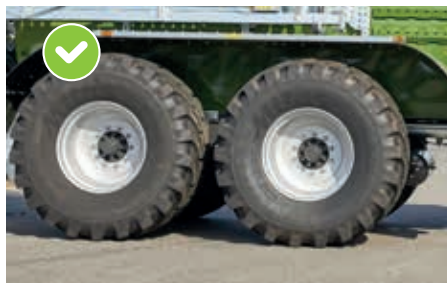
Wheel arch and tyres 750/60-R30.5" tyres Optional: 750/60-R30.5" tyres at rear, 850/50-R30.5 at front
