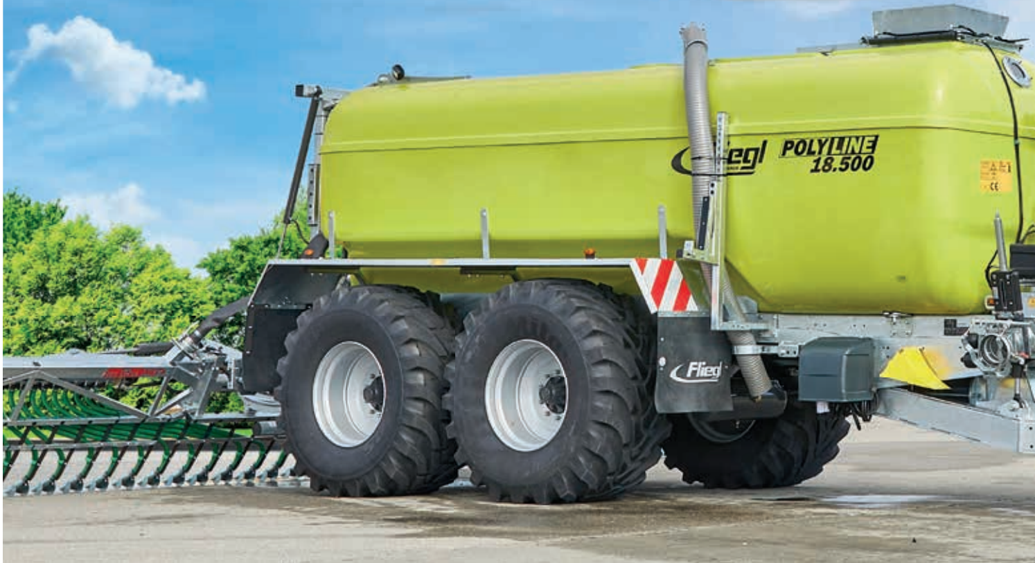
Pump tank Poly Line 900 with rotary piston pump
