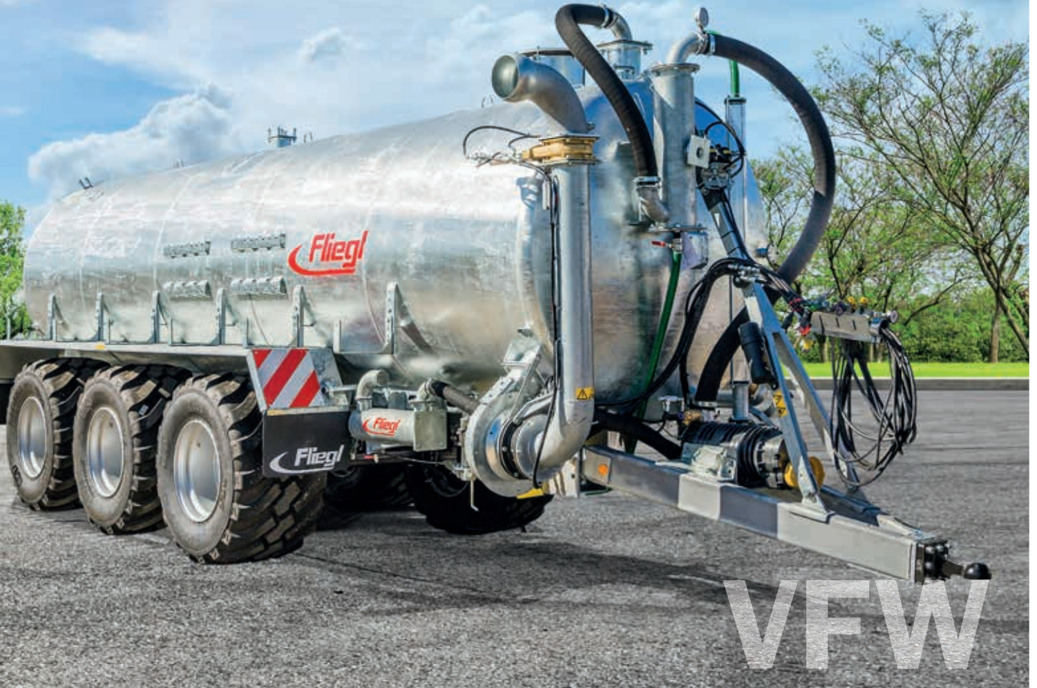
Only for vacuum tank: turbo filler with side-mounted quick coupler
