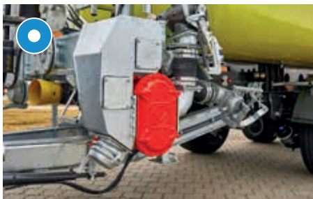
Very easy to maintain: mechanically operated rotary piston pump incl. reduction gear
