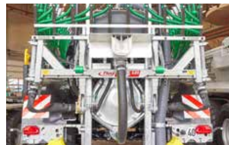
Additional spreading option with mounted baffle plate spreader
