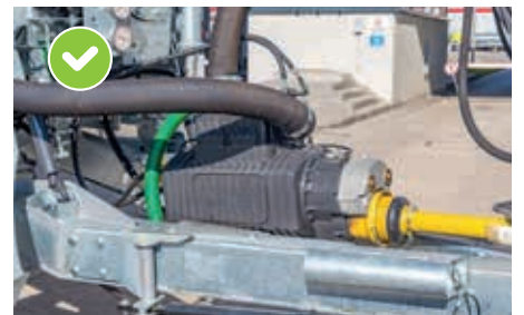
Heat-resistant compressor Optional: water-cooled compressor
