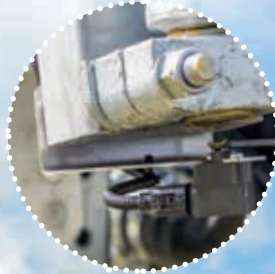
Angle sensors on left and right for uniform extension and retraction on slopes
