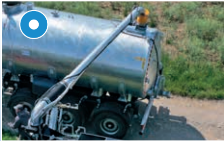
Only for pump tanks: 8" suction arm, 5 m length
