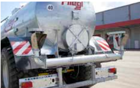
Double pendulum spreader, hydraulic
