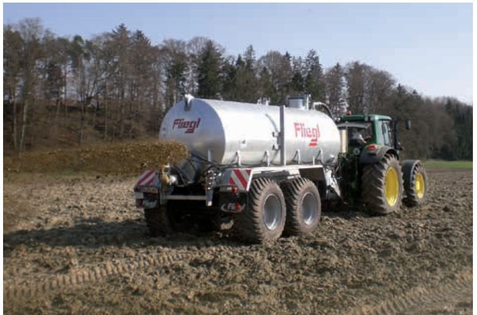
Pendulum spreader for coarse-droplet application
