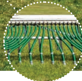
Even distribution quality with short outlet hoses
