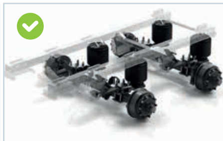
Air suspension Optional: hydraulic suspension
