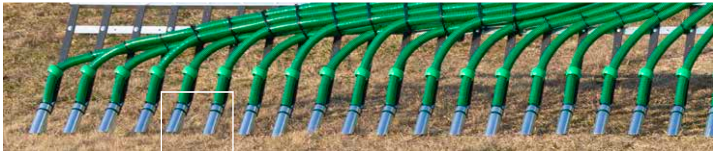
Shoe spacing of just 187,5 mm
