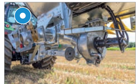
For vacuum tank: turbo filler positioned centrally under tank – for suction on either side
