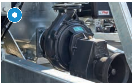
Centrifugal pump for transferring
