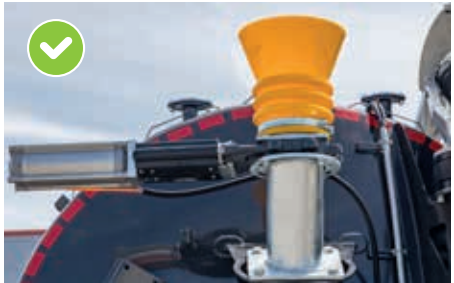
Rear docking funnel at top of tank
