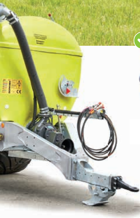
Elba centrifugal pump from Battioni, 3500 or 6500 l/min.
